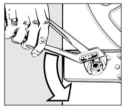
■ Using a pipe wrench turn the lefthand transit bar 90° anti-clockwise and the right-hand transit bar clockwise.
